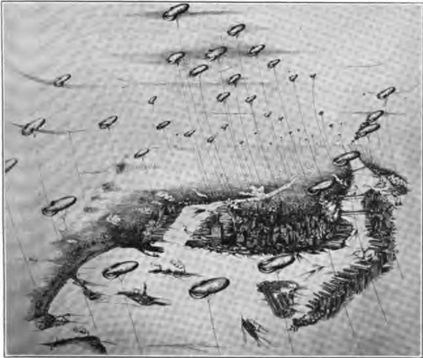
Diagram Illustrating Method of Protecting Large Cities by Barrage Balloons. Three Rings of Balloons Here Shown Surrounding New York City
