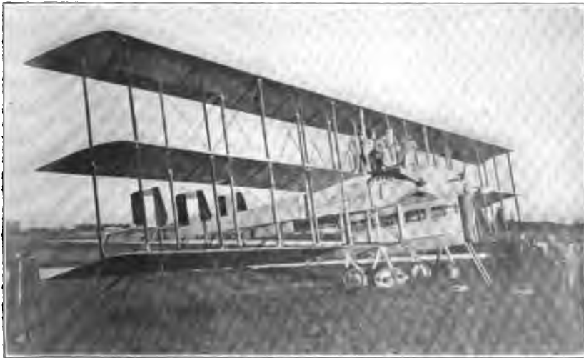
Italian Caproni Passenger Airplane. Carries About Fifteen Passengers and can be Rapidly Converted into a Bombardment Airplane
